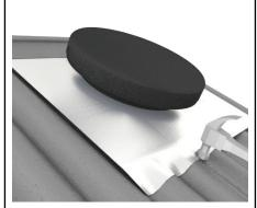
Gently form the top and bottom edges of tray to roof profile with a hammer or mallet.
