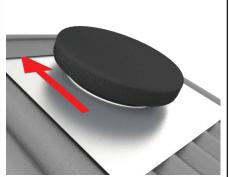
Position Roof Vent so the opening is located over hole in roof. Slide top of Tray under Ridge Capping if possible. \*Avoid installing over laps in sheets. If this cannot be avoided, you must use silicon to seal the laps from lowest point (soaker tray) to highest point of laps, ie: ridge cap.
