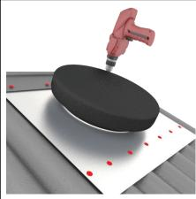
Using Tech Screws, screw the Soaker Tray into Ridge Capping and top of corrugations.
