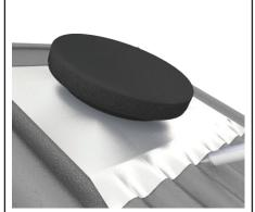
Seal under all edges of soaker tray to roof with silicon.
