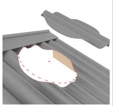
Using a drill, mark the centre point in the roof for Roof Vent location.
